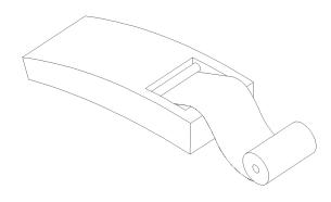
Put the paper roll at the back of the device (See draw) Introduce the paper under the cylindrical paper driver. Maintain a light pressure on the paper, press the paper feed (1). Ensure you a good guidance of the paper. Put the paper roll in its compartment and strongly push it downwards. You will feel a click as soon as the paper roll will finds its housing.
