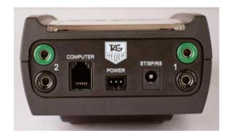
**INPUTS 1 & 2** Inputs for timing impulses.
