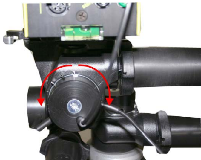
ROLL – level the camera horizontal (see spirit level)
